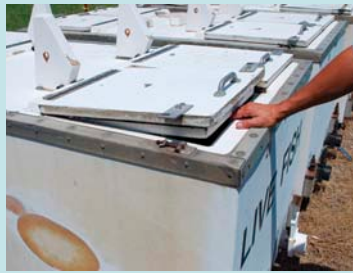
Photos 1 (left) and 2: The lids of live tanks on hauling trucks can fall if the truck moves. One farmer used pneumatic hinges to eliminate the hazard.
